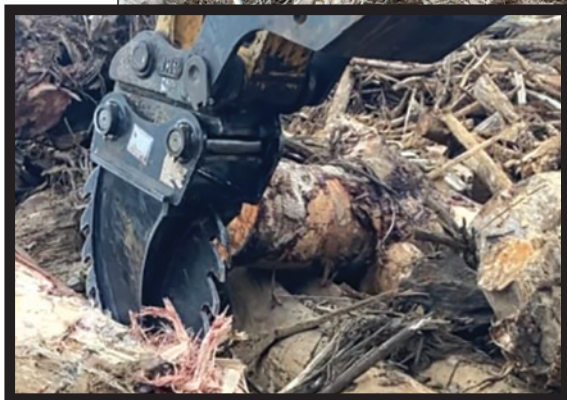
The Ransome Shark Tooth stump splitter/harvester was mounted on a mid-size excavator to size down logs and stumps for processing by the Crambo 6000 dual-shaft shredder.
